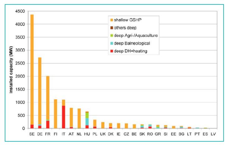
Figure 2 – Distribution of installed capacity (MWth) in EU 27 member states (after data from WGC, 2010; EurObservER, 2011; EGEC, 2011)
